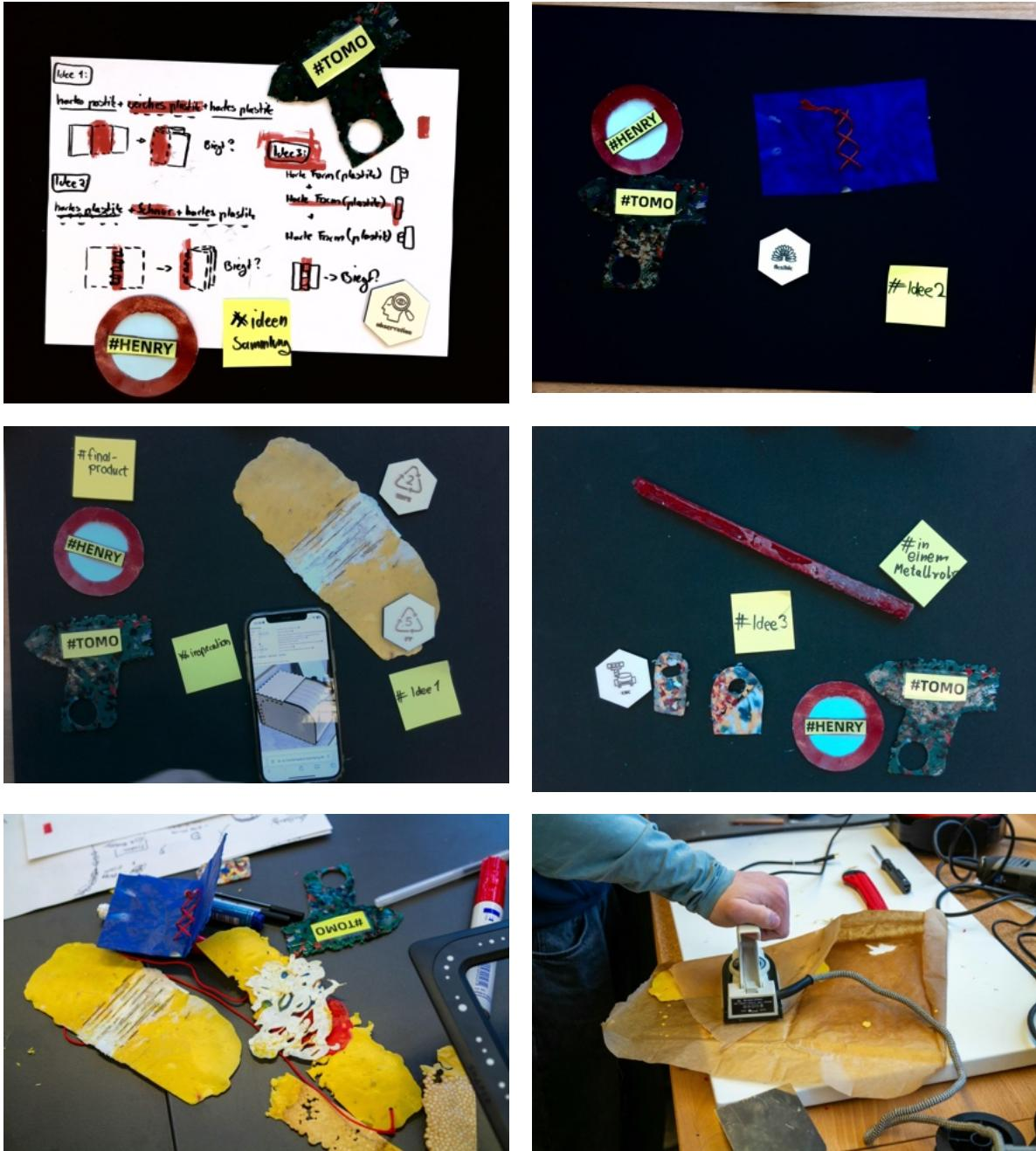
*Note.* This group was dealing with various mechanisms, bending plastics for repeating purposes. They acted planfully, sketching initial ideas and doing all material testing necessary to evaluate different techniques. *Image Credit: Photos by the author.*
