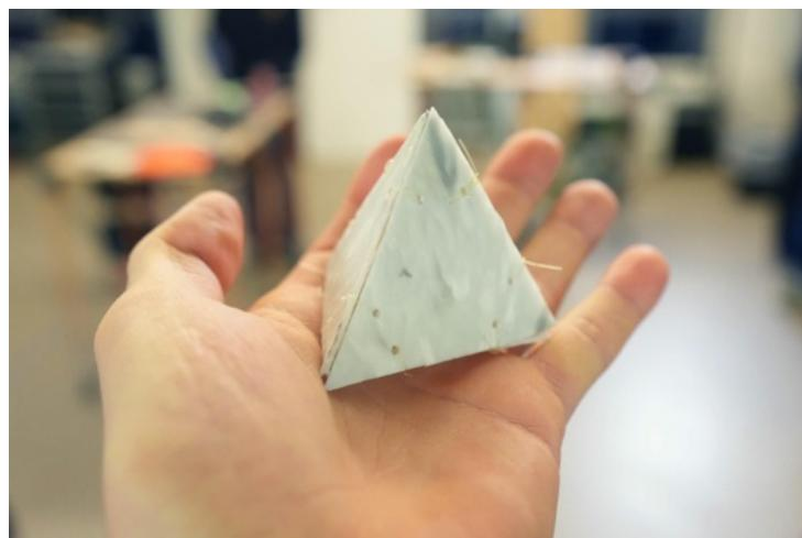
*Note.* A Pyramid served as the first test in exploring whether sewing plastics is a feasible option for flexible hinges. Combining different materials and properties in a reversible way is a skill the industry lacks. Many recycling steps can majorly benefit from adjustments made in the design phase. Consider as example the multilayered Tetra Pak packaging material, in contrast to the yogurt packages where the paper packaging could be removed tool-free. *Image Credit:* Beril Ece Güler / InKüLe
