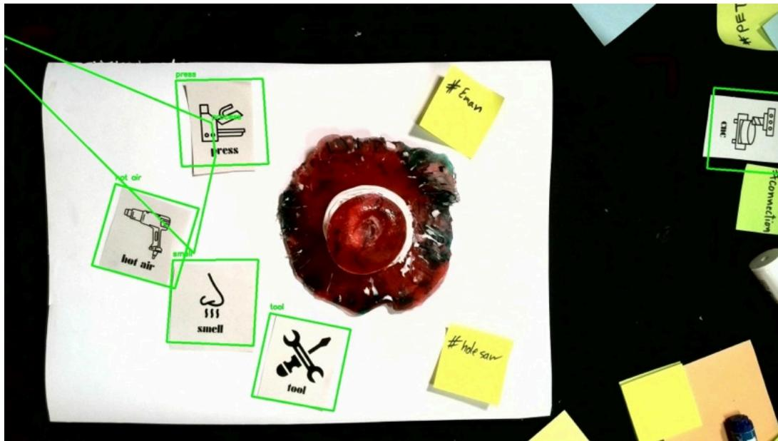
*Note.* In this image, the detected templates are visualized with bounding boxes as overlay. As visible, the process is not completely reliable (see the false positive template drawn), but it can handle rotation, partly occluded markers and slight perspectival shifts. Several optimizing customizations were implemented, like assuming all markers are square and have a certain size, which helps discarding false positives. *Image Credit: Photo by the author.*
