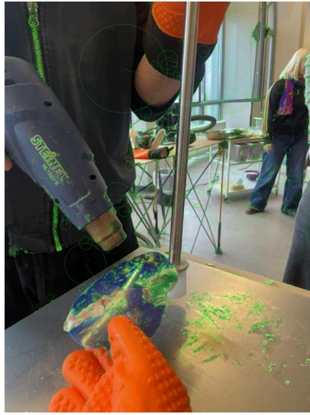
*Note.* A view with one of the internal template matching algorithms visible as overlay. It first detects edges and salient keypoints, usually areas of high contrast, then compares those against a set of known images, the markers. The visible circles were created using the ORB algorithm via openCV (OpenCV Contributors, 2012). *Image Credit: Photo by the author.*
