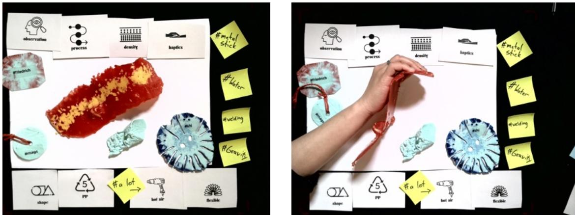
*Note.* Here, the Workshop participants explored ways to form a sheet of plastic to a hand shape. As can be deducted from the markers, that was done with a variety of tooling, notably trying out the heat-resistant silicone gloves, using them under the heat guns to obtain real forms of the hand.
