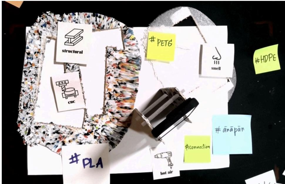
*Note.* A participant used the CNC options to create a smartphone stand from multiple fabricated sheets of plastic. As seen in the documentation of it, PLA and PET were used here, two especially strong materials that delivered good results while being cut. The connections and joints are reminiscent of typical laser-cut connections.
