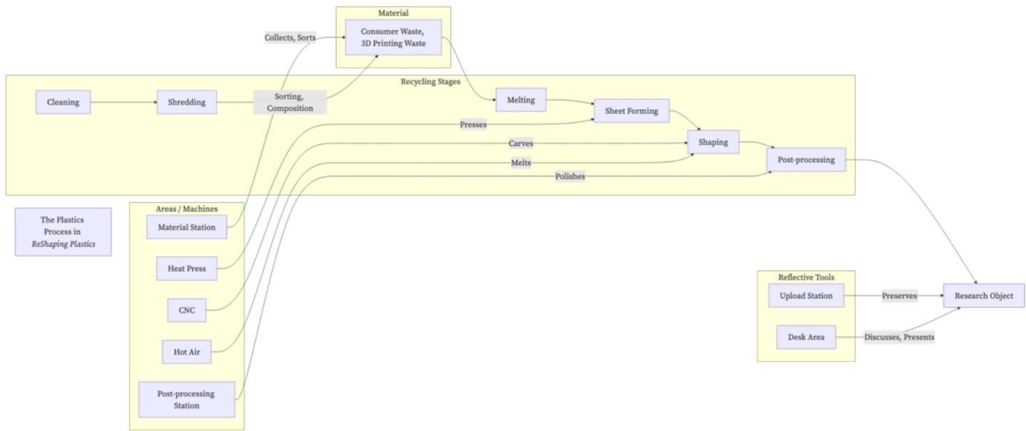
*Note.* Plastic recycling is a complex, multi-step process. It involves several stages, and on an industry scale, many different pathways are established. For a good overview of different industrial pathways see Volk et al. (2021). Presented for this work is an adapted workflow that incorporates feasibility in smaller scales and is designed with the machinery and PPE process at hand in mind. *Image Credit: Graph by the author.*
