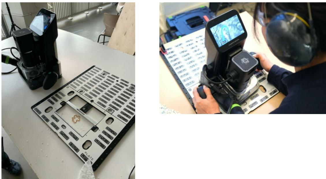
*Note.* The Shaper Origin combining digital and analogue fabrication techniques. It is of special interest in education contexts, because various self-checks and correction features make usage much more accessible than a traditional, purely computer-controlled CNC-Machine.
