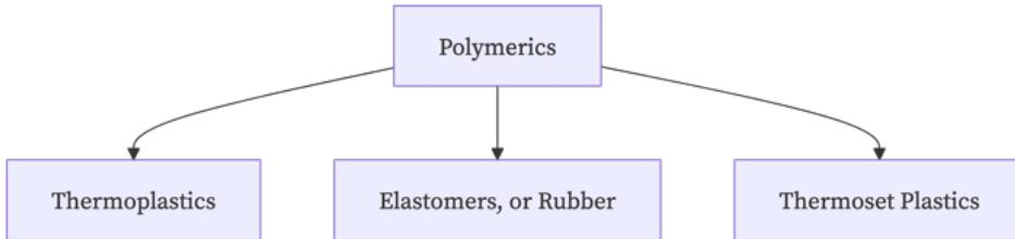
Note. Sometimes one finds elastomers excluded from this overview, as they are not necessarily a polymer. It is more of a functional definition: anything that stretches, is an elastomer. It can be of thermoplastic origin, then it is a thermoplastic elastomer (TPE), but it can be another class altogether, much like vegetables do scientifically speaking not really exist (Katz, 1998; Precious Plastic, 2025). *Image Credit: Graph by the author.*
