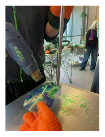
*Note.* A view with one of the internal template matching algorithms visible as overlay. It first detects edges and salient keypoints, usually areas of high contrast, then compares those against a set of known images, the markers. The visible circles were created using the ORB algorithm via openCV (OpenCV Contributors, 2012). *Image Credit: Photo by the author.*
