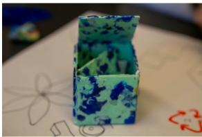
*Note*. These two were constructing a plastic box from a single sheet of plastic, borrowing sheet-bending techniques from metal. They were also developing a technique where they patterned the plastics in the molten state to get leafy structures. *Image Credit: Photos by the author.*
