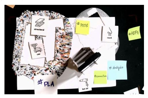
*Note.* A participant used the CNC options to create a smartphone stand from multiple fabricated sheets of plastic. As seen in the documentation of it, PLA and PET were used here, two especially strong materials that delivered good results while being cut. The connections and joints are reminiscent of typical laser-cut connections.
