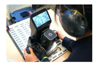
*Note.* The Shaper Origin combining digital and analogue fabrication techniques. It is of special interest in education contexts, because various self-checks and correction features make usage much more accessible than a traditional, purely computer-controlled CNC-Machine.
