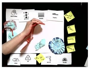
*Note*. Here, the Workshop participants explored ways to form a sheet of plastic to a hand shape. As can be deducted from the markers, that was done with a variety of tooling, notably trying out the heat-resistant silicone gloves, using them under the heat guns to obtain real forms of the hand.
