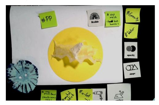
*Note*. Results from a group examining thermoforming properties of different plastic types. This piece was from some leftover foodstuffs box tops, that was then successfully identified using density testing methods supplied in the workshop and shaped with the heat gun and a water bath. Image location in the archive Image Credit: Photo by the author.
